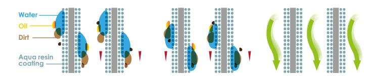
The new SHORAI R32 model range comes equipped with a self-cleaning indoor coil function. This new control reduces the moisture build up on the coil and inhibits the formation of any mould. Using a combination of a specially-coated aluminium coil that will not allow condensation to form and an internal fan, which will continue to run for a specific amount of time even after the units has turned off, ensures long lasting performance and a high quality air environment.
